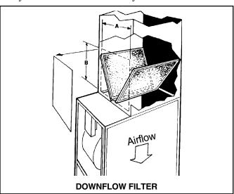
A downflow/horizontal furnace return air filter application, as shown, features two 14" x 20" x 1" filters in the 17-1/2" wide furnace cabinets; or two 16" x 20" x 1" filters in the 21" and 24-1/2" wide furnace cabinets.
