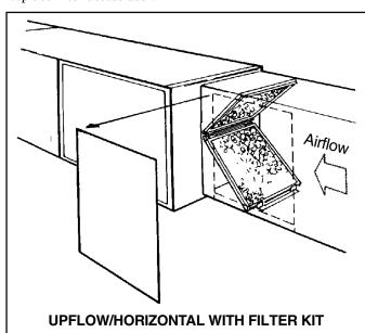
Air filters may also be located outside of the furnace using a remote filter grille. The filter grille could be in a hallway, wall, or in the ceiling. Check with your dealer for the exact location of your filter and the method of changing the filters.
