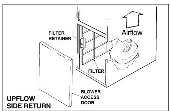
For vertical UPFLOW ONLY, a left or right return air inlet as above (left side shown) requires trimming of the factory supplied filter to 17" x 25" x 1" for both the 21" and 24-1/2" wide furnaces.
